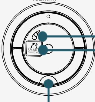
A spring-loaded swivel cap covers a smart charging dual USB port on top of the unit
