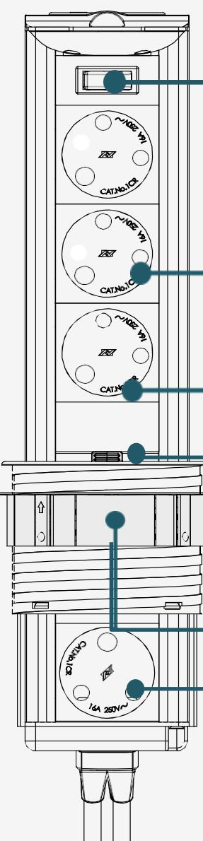
15A thermal overload switch protects the unit from power overloads
